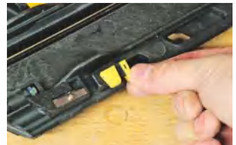
Spare soft-nose tips are supplied and stored on board with each gun
